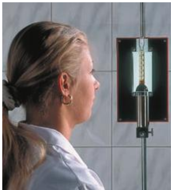
Fig. 6 Measured values can be reliably and accurately read off with the aid of a safety reading lamp
